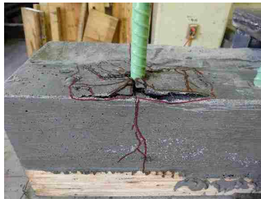
Figure 6.4. Breakout deformations observed after testing splice-connection curb specimens.
