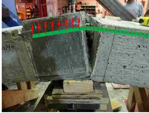
Figure 7.8. Upward force distribution from bent reinforcement.
